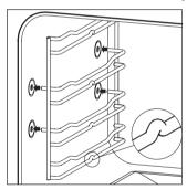
■ Make sure that they are correctly inserted when replacing them (see illustration). Push the runners in firmly.
